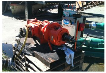
Place: Sludge type: Equipment: Treated volume: UTE EDAR Butarque (Madrid) High solids sludge from an anerobic digester in a WWTP Mobile unit up to 90 m<sup>3</sup>/h, long conveyor and extraction set 9.000 m3
